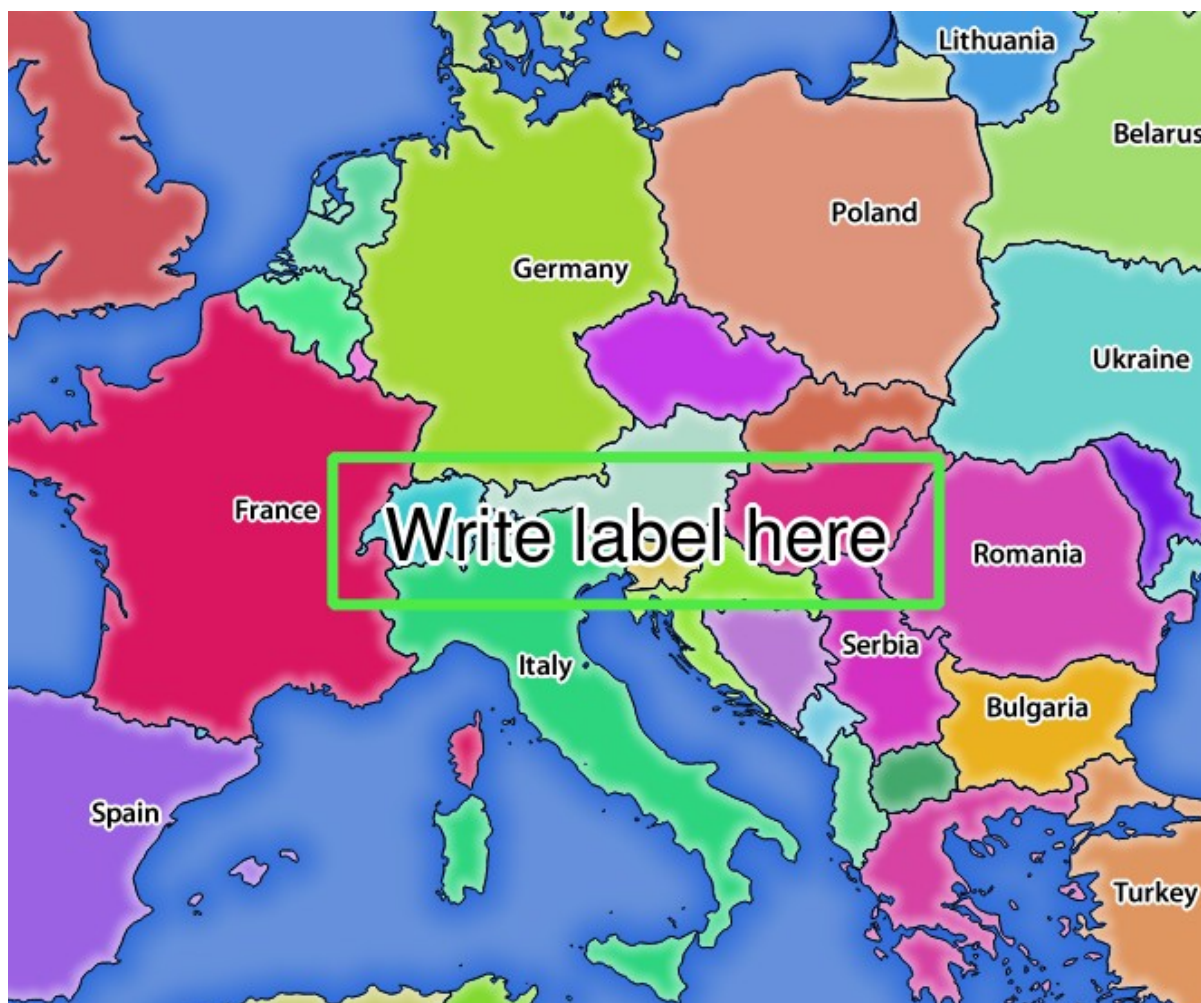
图 3.7: Server response to a GetMap request with redlining parameters
