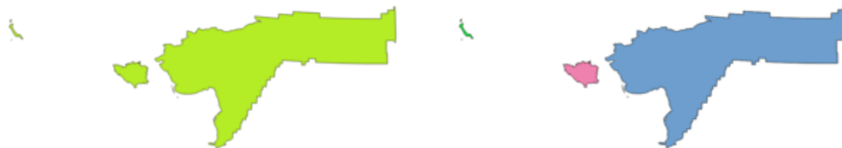
Şekil 24.69: Left the multipart source layer and right the single part output result
