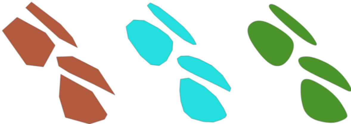
Рис. 24.81: Increasing number of iterations causes smoother geometries
