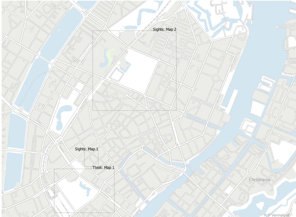
Рис. 11.13: Example of layout extents displayed in a QGIS project with two print layouts. The print layout named „Sights“ contains two map items, while the other print layout contains one map item.
