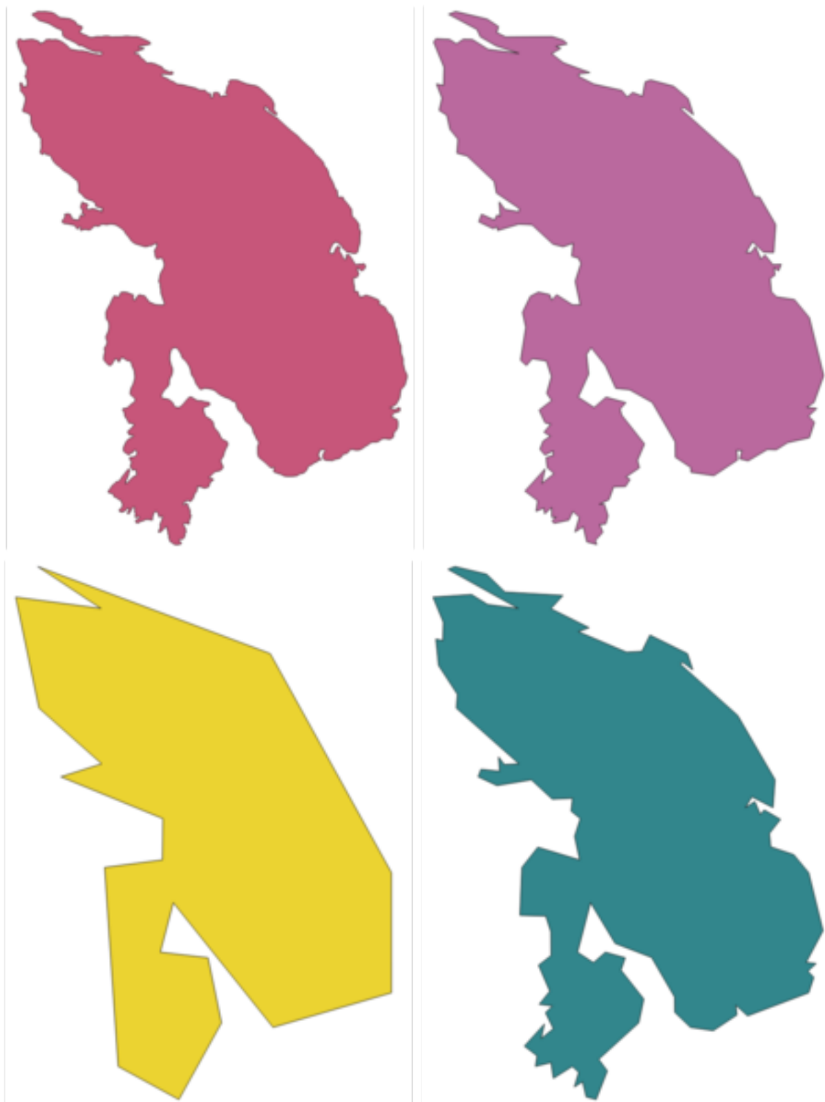
Рис. 24.79: Clockwise from top left: source layer and increasing simplification tolerances
