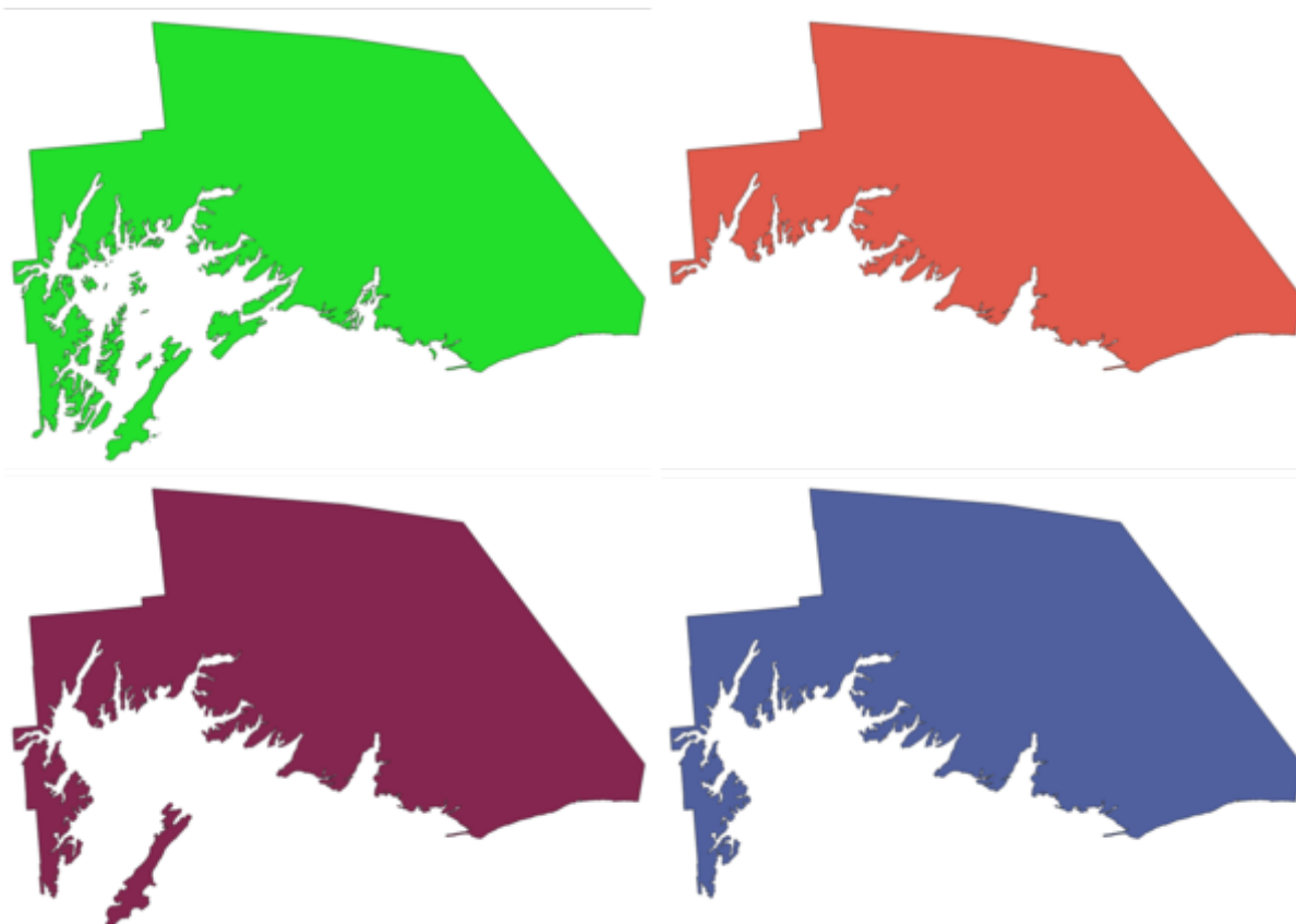
Fig. 24.64: Clockwise from top left: original multipart feature, one, two and three biggest parts kept
