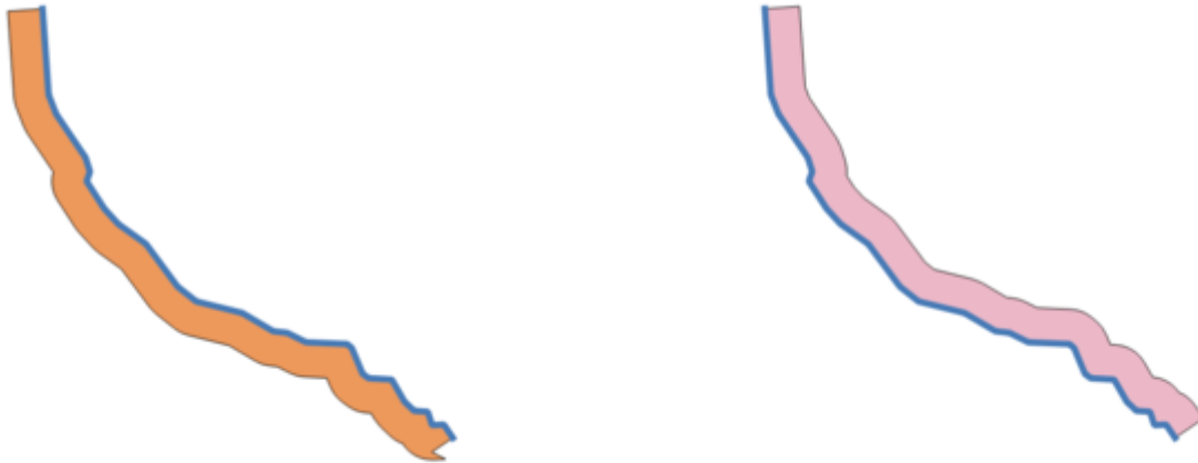
Fig. 24.80: Left versus right side buffer on the same vector line layer
