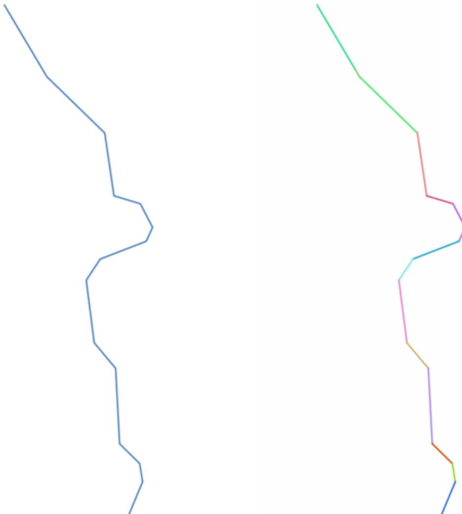
Fig. 24.58: The original line layer and the exploded one
