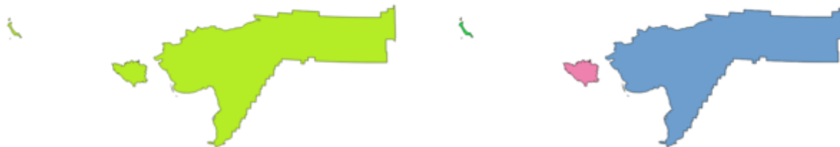
Fig. 24.69: Left the multipart source layer and right the single part output result
