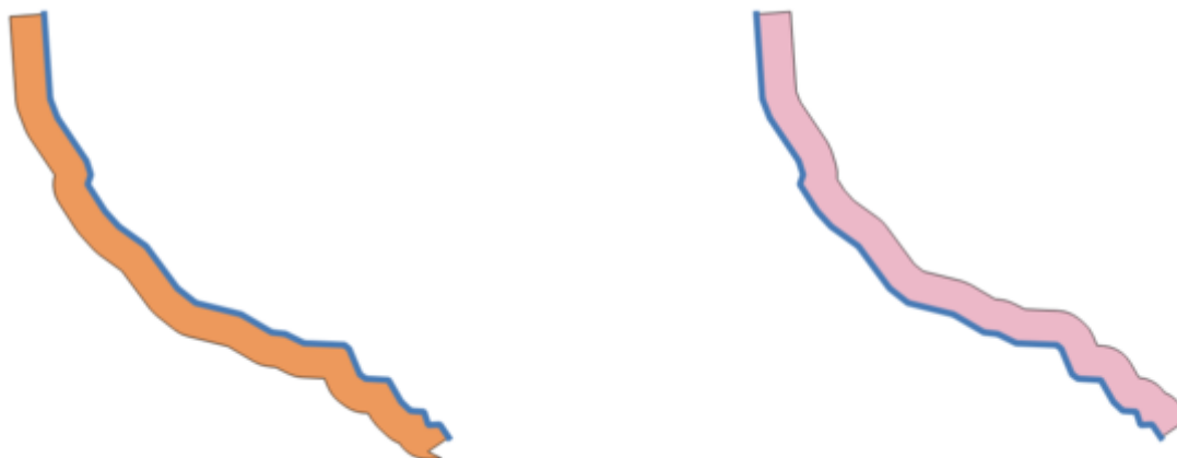
24.80. ábra: Left versus right side buffer on the same vector line layer
