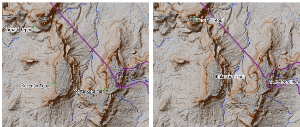
Abb. 24.40: Vector point layer (green dots) before (left), and after (right) an affine transformation (translation).
