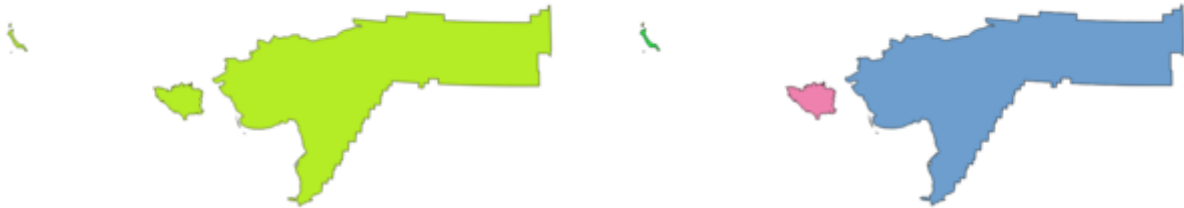
Obr. 24.69: Left the multipart source layer and right the single part output result
