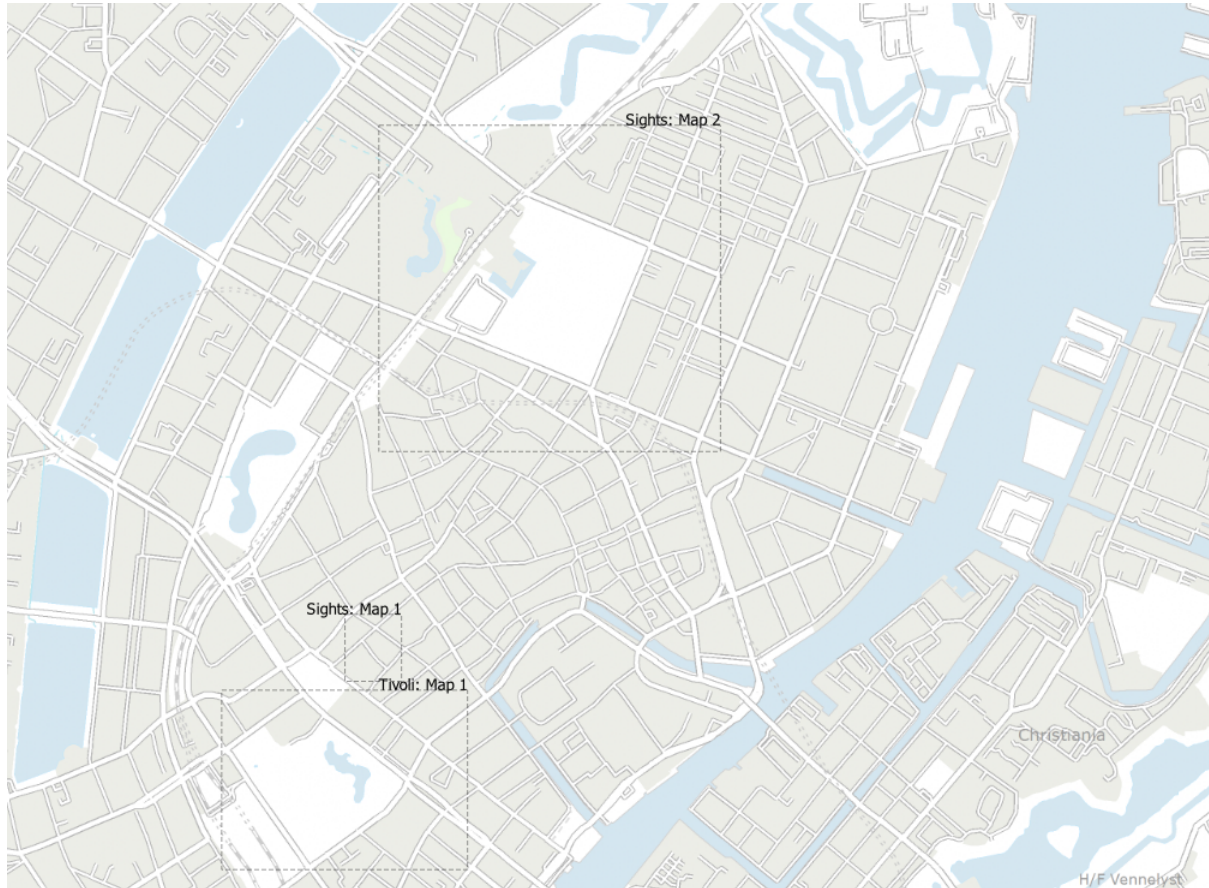
图 11.13: Example of layout extents displayed in a QGIS project with two print layouts. The print layout named 'Sights' contains two map items, while the other print layout contains one map item.
