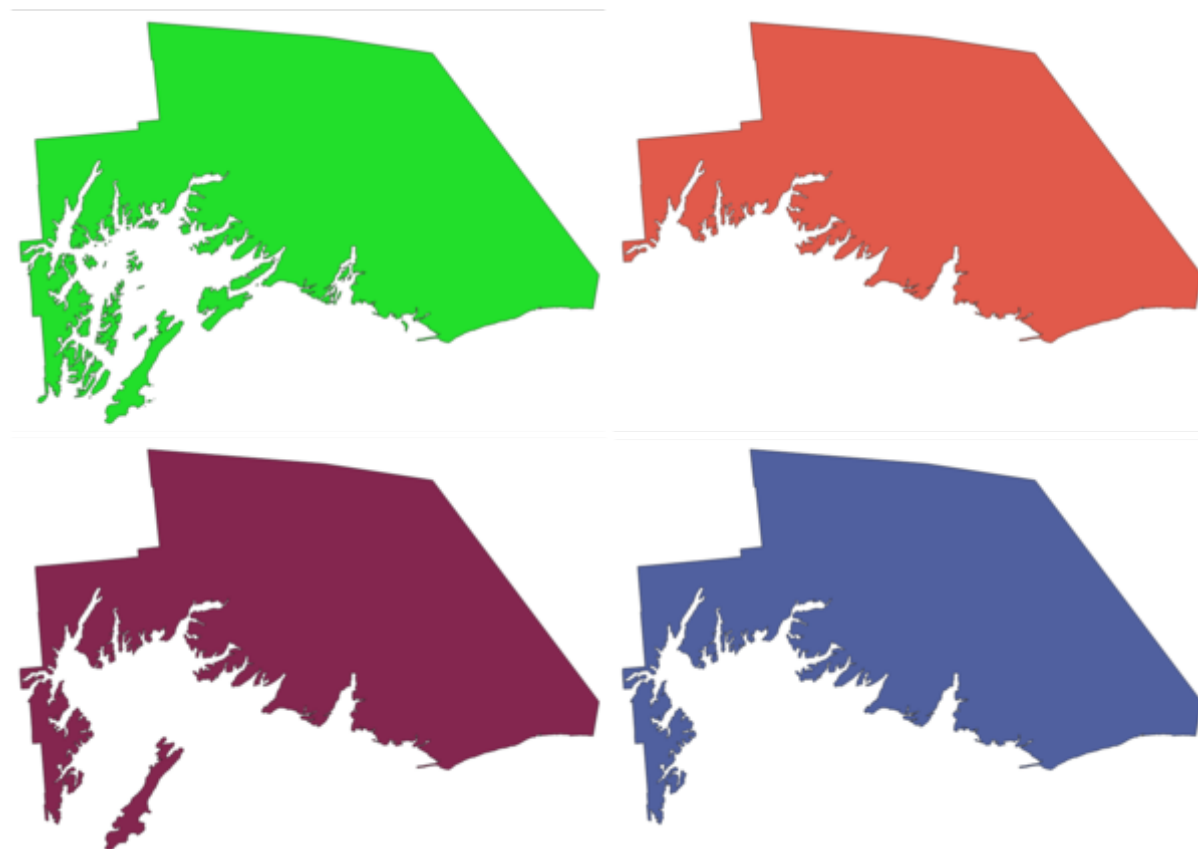
图 23.49: Clockwise from top left: original multipart feature, one, two and three biggest parts kept
