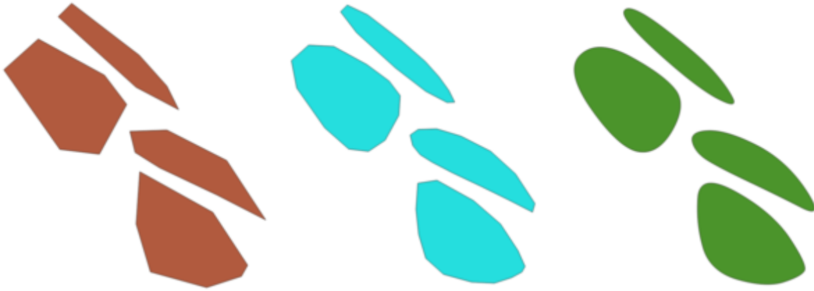
图 23.67: Increasing number of iterations causes smoother geometries
