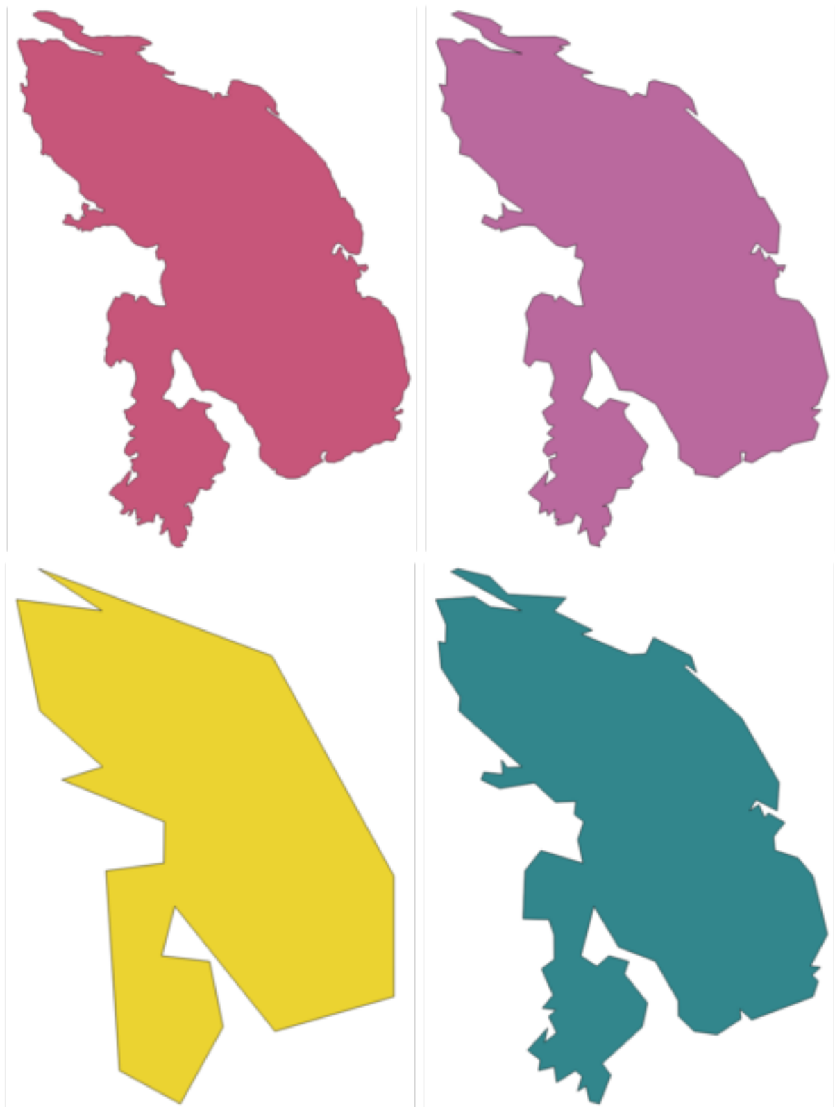
图 23.65: Clockwise from top left: source layer and increasing simplification tolerances
