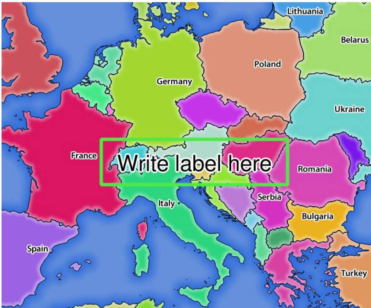
图 18.14: Server response to a GetMap request with redlining parameters
