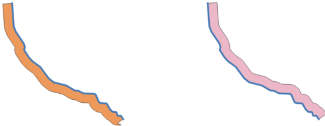
图 23.66: Left versus right side buffer on the same vector line layer
