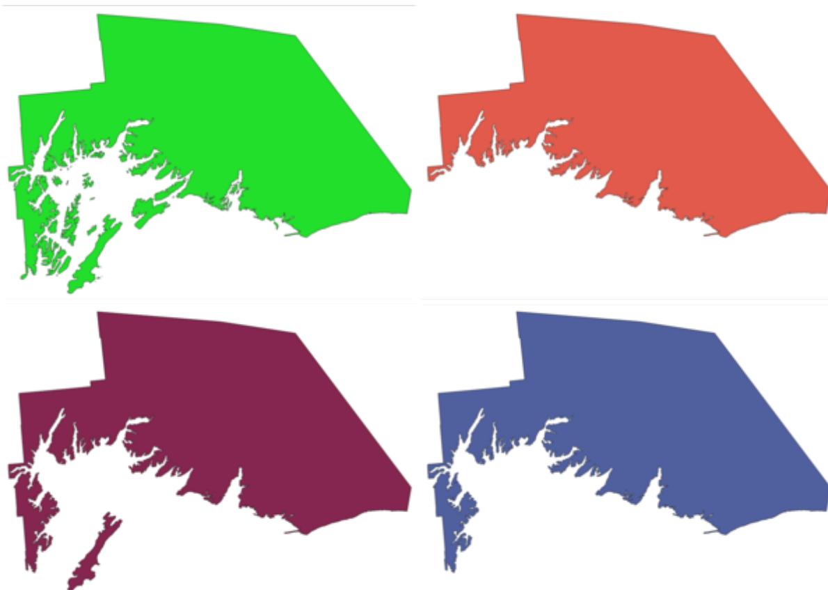
Şekil 23.49: Clockwise from top left: original multipart feature, one, two and three biggest parts kept
