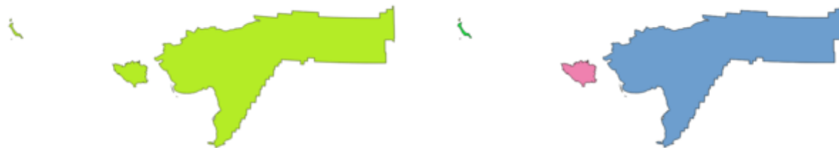
Şekil 23.54: Left the multipart source layer and right the single part output result
