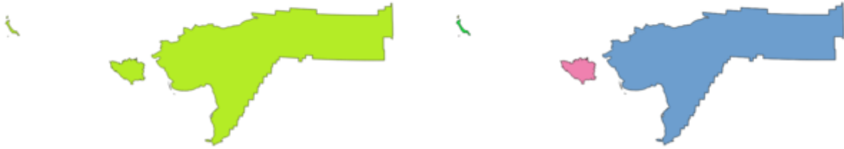
Fig. 23.54: Left the multipart source layer and right the single part output result
