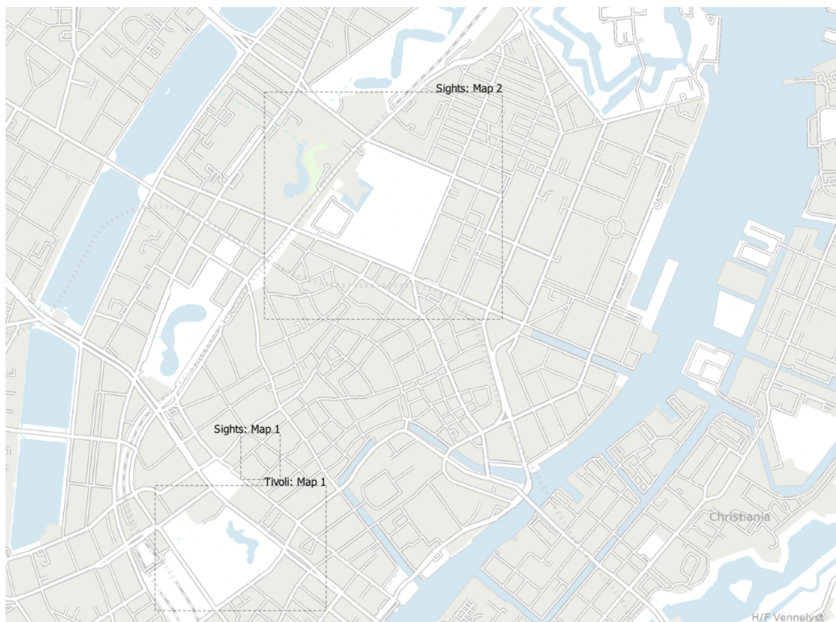
Fig. 11.13: Example of layout extents displayed in a QGIS project with two print layouts. The print layout named 'Sights' contains two map items, while the other print layout contains one map item.
