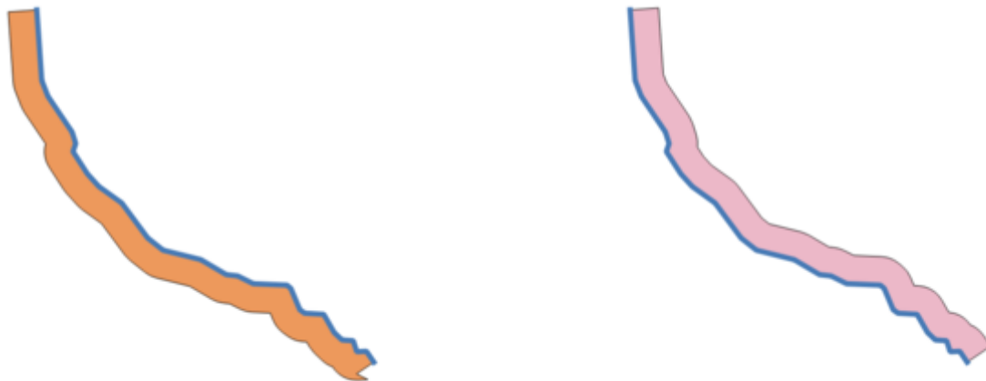
Gambar. 23.66: Left versus right side buffer on the same vector line layer
