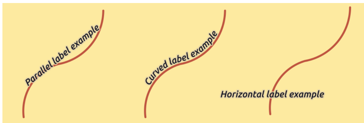
Gambar. 12.20: Label placement examples in lines
