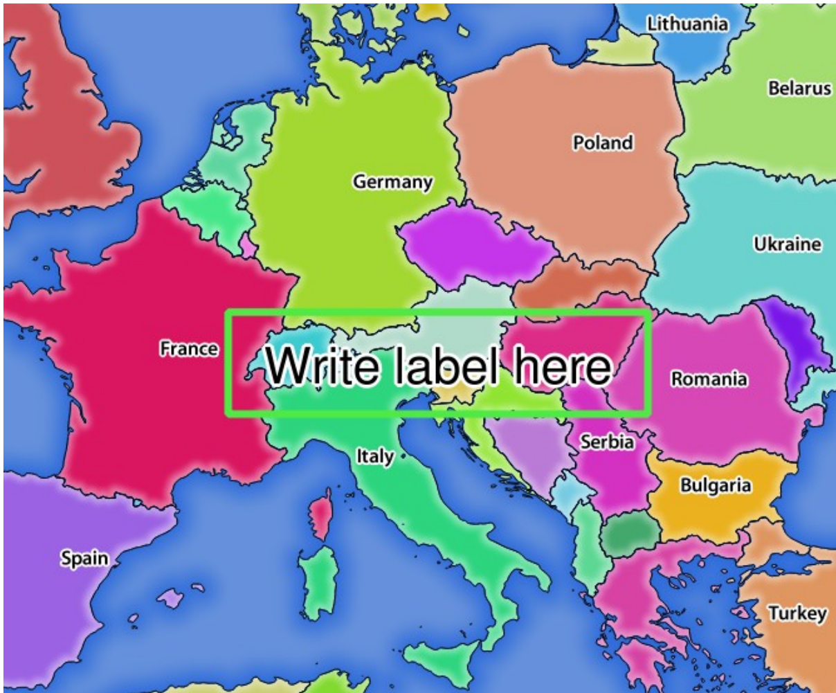
Figure 15.7: Server response to a GetMap request with redlining parameters
